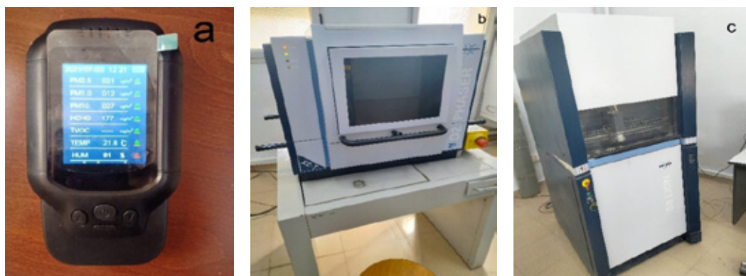
Figure 4. Equipment used in the quantitative and qualitative analysis of dust emitted from the quarry (a: The air quality meter: a multifunctional air quality-measuring device PCE-RCM 8. Brand: Fambasis, b: Benchtop X-ray diffractometer BRUKER D2 PHASER, and c: Fluorescence spectrometer S8 LION, dispersive X-ray machine Bruker AXS (manufactured in Germany)
